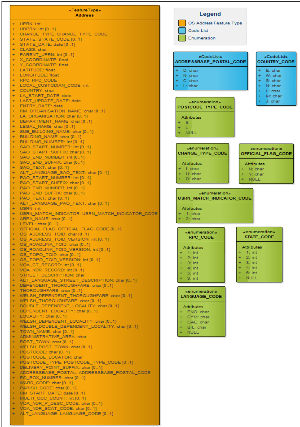
Figure 2: UML model showing AddressBase Plus feature types, enumerations and code lists for the CSV supply
