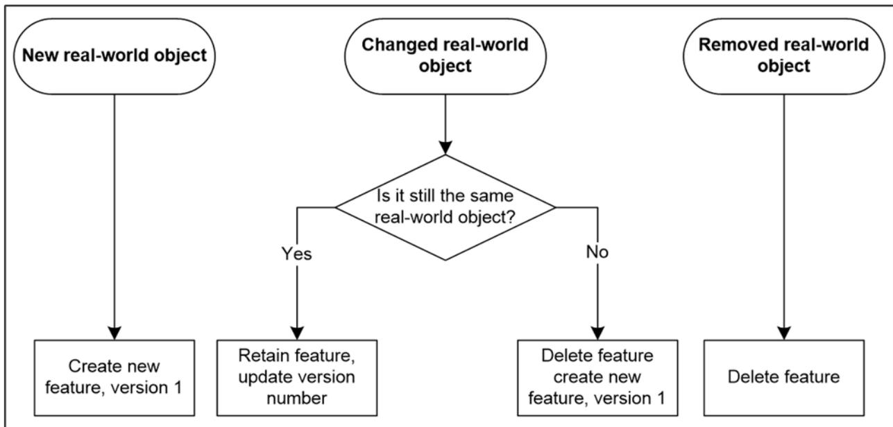
Figure 6: Polygon feature creation process in OS MasterMap Topography Layer.
