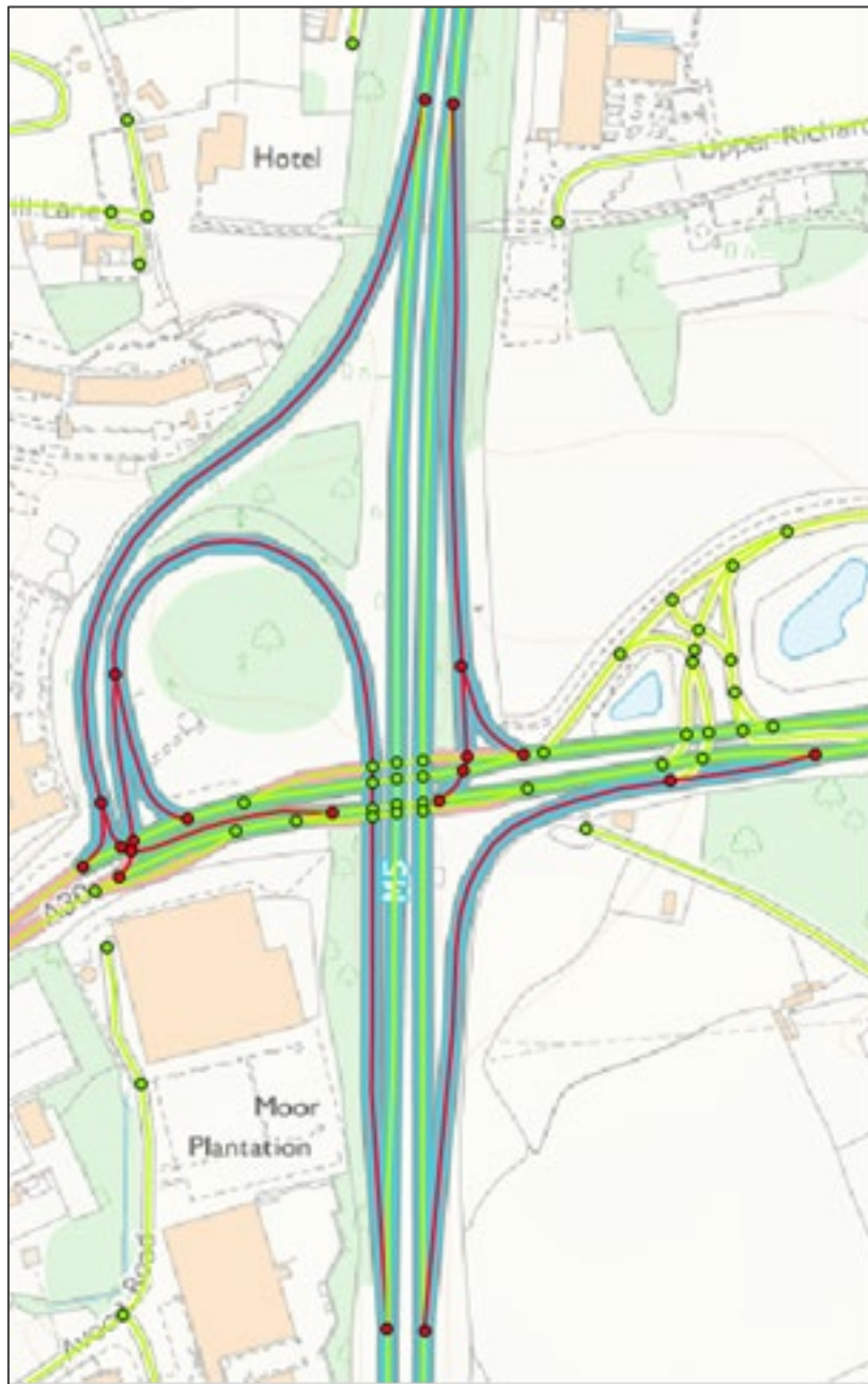
Figure 12. Collection of RoadNodes making up a road junction (highlighted red). RoadLinks representing the slip road are highlighted red for clarification only.
