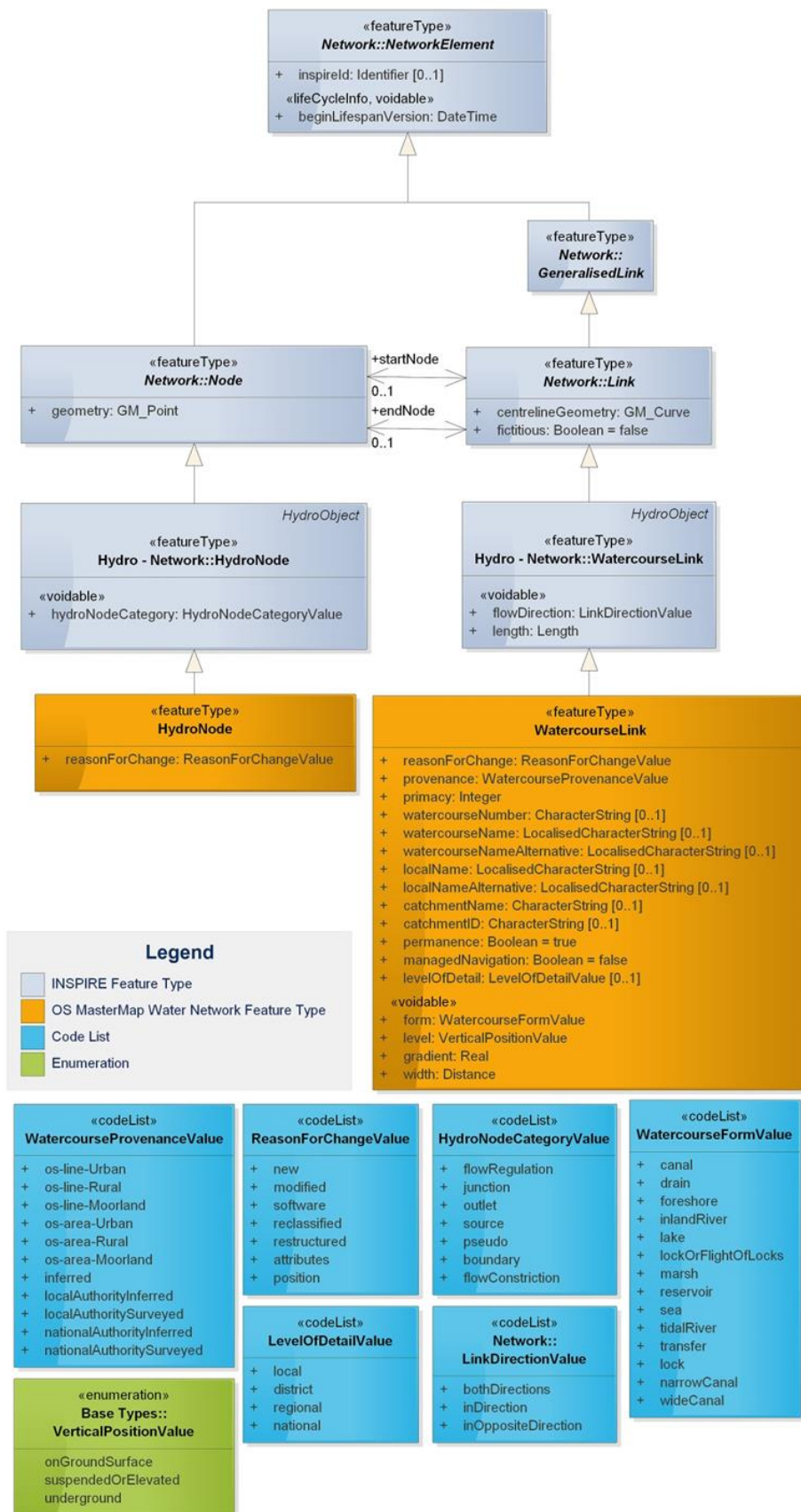
Figure 4: UML diagram showing the data structure of OS MasterMap Water Network Layer in the current release.
