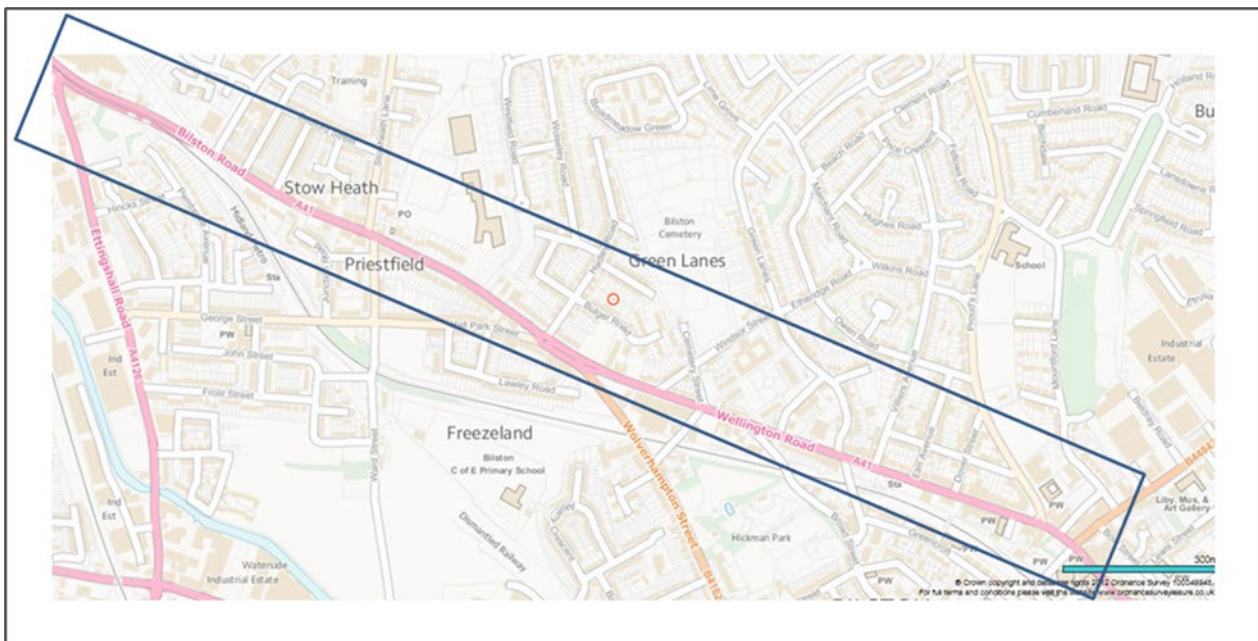
Figure 5. A Road feature references all the Road Links that represent a numbered road, for example, the A41.
