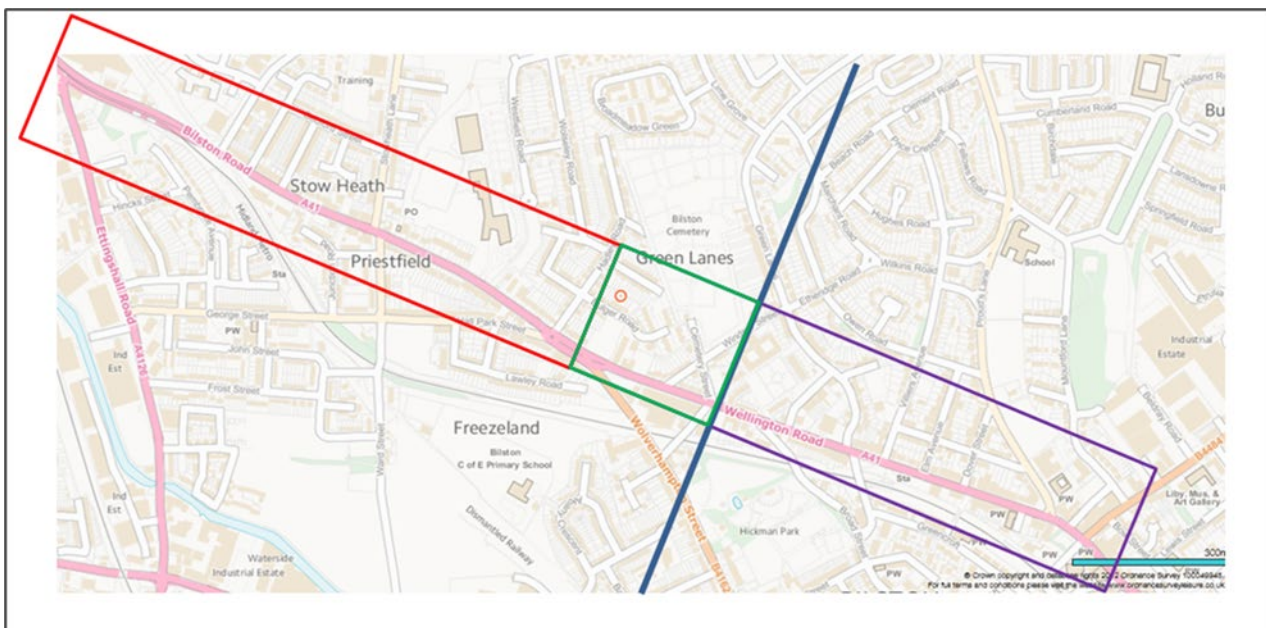
Figure 6. Where a named road crosses an administrative boundary, a new Street feature will be created, as can be seen in the above example for Wellington Road.
