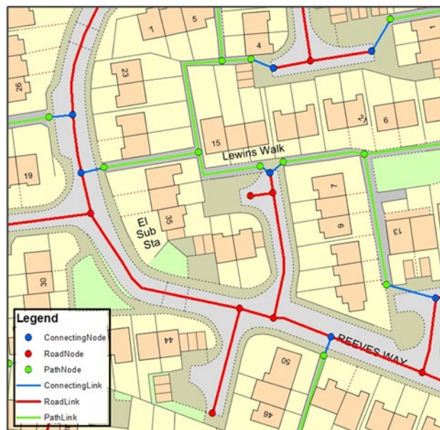
Figure 3. How Connecting Links and Connecting Nodes connect the road and path networks together. Connecting Nodes are coincident with Road Nodes.
