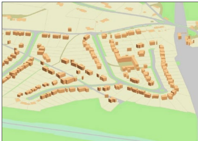
Figure 2: Map of the same area which has been generated using OS MasterMap Topography Layer – Building Height Attribute. The buildings and structures are in 3D.
